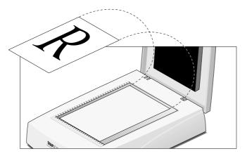
The optical performance of a CCD scanner is always best near the middle of the glass plate. However, the specified scan quality is guaranteed for the entire scan area. If you put more than one original on the glass plate, position them as close to the center line as possible to optimize the quality.
